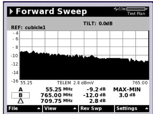
Forward sweep uses a unique referencing method to accurately reveal any problems in the system without interfering with any of the analog or digital carriers.
