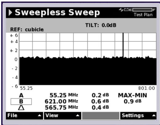
Sweepless Sweep provides a quick method to check cable system integrity using active channels to sweep the forward path. Sweep points do not need to be added and no forward-path headend gear is required.
