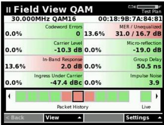
The Field View QAM dashboard shows a variety of measurements for the represented carrier, and results that are outside of user-designated limits are indicated by color. From the dashboard, technicians can select a measurement parameter to view more closely and switch directly to a full-screen display of that measurement.
