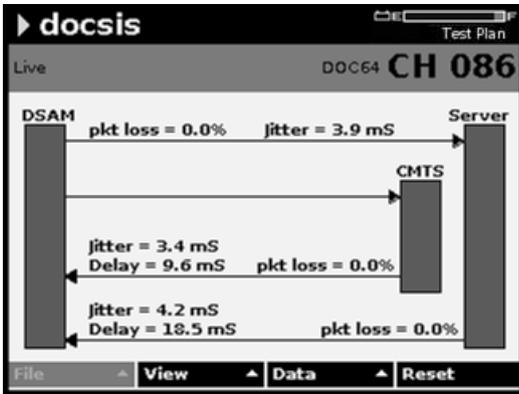
The VoIPCheck voice-quality verification test runs over the DSAM's cable-modem DOCSIS connection. It allows for segmentation between HFC and IP issues by showing at which side of the CMTS data impairments are present.
