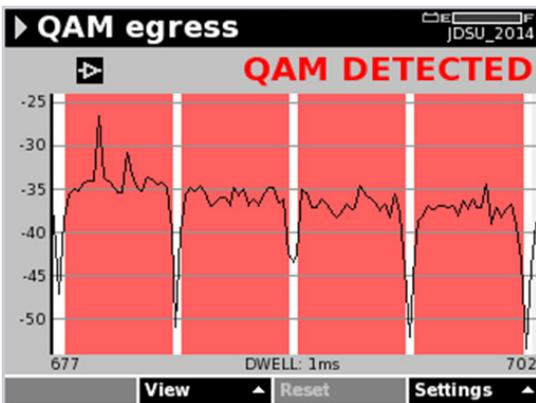
The QAM Egress option simplifies the detection of leaks (and verifying fixes) identified by leakage monitoring systems.
