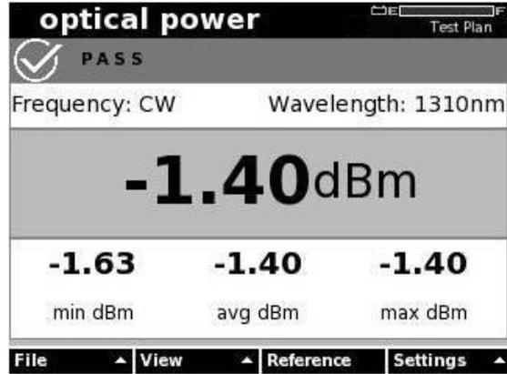
The optical power measurement option enables connecting a USB power meter (JDSU MP60A or MP80A) for verifying or troubleshooting node light levels.
