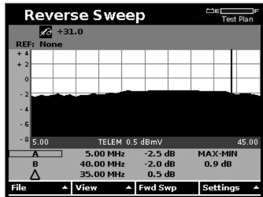
Tight reverse sweep points in the sweep plan display the entire return path with better resolution and help to find mismatches or other problems in the upstream transmission path.
